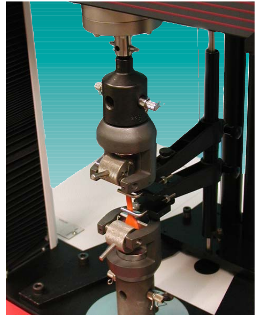
▲ Rubber test on a dual column
