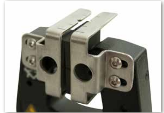
Jaw Face Shields reduce pinch hazards and have useful specimen alignment features
